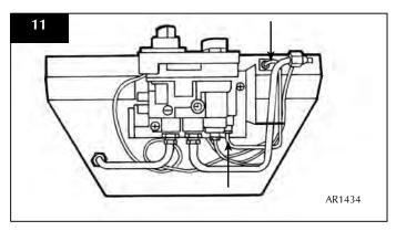
• Remove the pipe and the injector drops out from the pilot unit. Take care not to loose or damage the injector.
